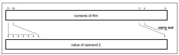
Figure 4-8: Arithmetic shift right
