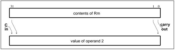
Figure 4-10: Rotate right extended
