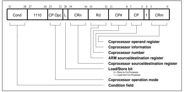
Figure 4-27: Coprocessor register transfer instructions
