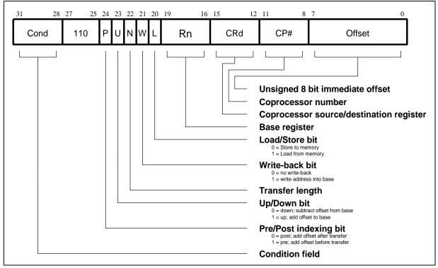
Figure 4-26: Coprocessor data transfer instructions
